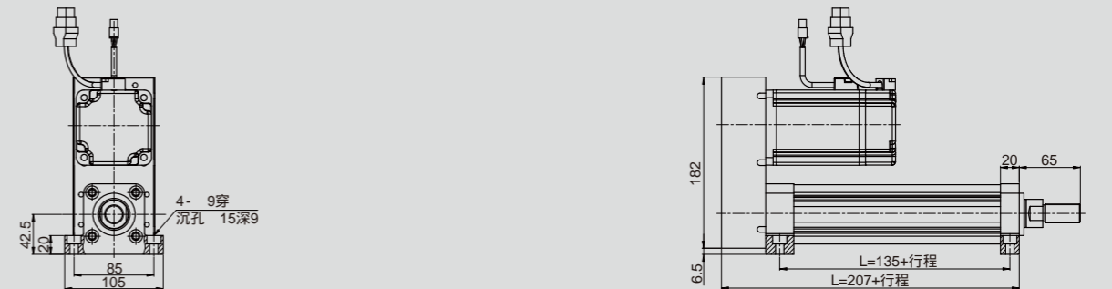
LOE50轉折側面安裝-LA LOE50Transition Side Installation-LA
